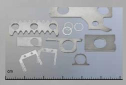
Laser-cut parts of all sizes can be manufactured to precision within a hundredth of a millimetre
